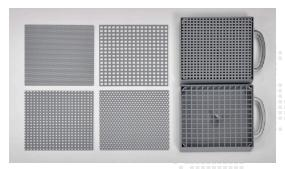
Given the importance of paw tactile sensitivity in rodents, while the design of commercially available CPP boxes has traditionally focused only on the wall patterns and colors, the Ugo Basile CPP box includes 4 interchangeable floors with different patterns & texture.
