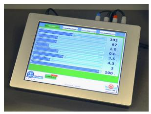
The Unit, incorporating a 12" touch-screen, manages the Passive Avoidance Test via the **40550-010** Software. Up to 4 cages can be connected to the same Controller.
