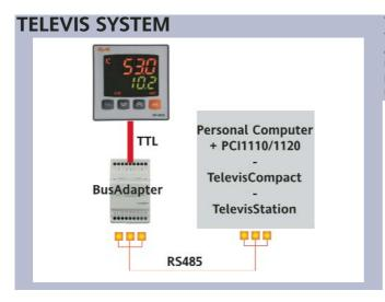
The device can be connected to Televis remote control systems through a TTL serial port (use TTL- RS interface module 485 BUS ADAPTER 130 or 150) or, in models where provided for (EW4822), by means of direct RS485 connection. To configure the device for this purpose, open the folder identified by the "Add" label and use parameters "dEA" and "FAA".
