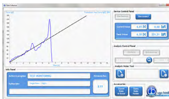
Figure 1: Screenshot of the GSM software showing the force trace (in red) and the desired target force rate (in blue) - slope function
