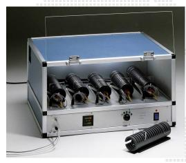
The **58000-850 Rat Scanner** is also available, combining the pre-warming features, with an electrical/pneumatical switch which enables connection of up to 5 rodents, tail cuff and pulse pick-up positioned on their tail, to scan their blood pressure in sequence.
