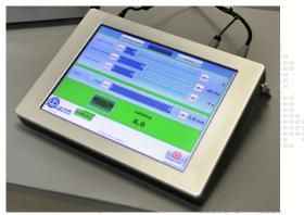
The Unit, incorporating a 12" touch-screen, manages the Passive Avoidance Test via the 40570-010 Software. Up to 4 cages can be connected to the same Controller.
