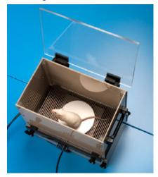
The detachable circuplatform, lar diam. 7cm, is positioned at the centre of the cage, on protruding а stud fastened to the actuator, the mechanism which energizes the platform vibration.
