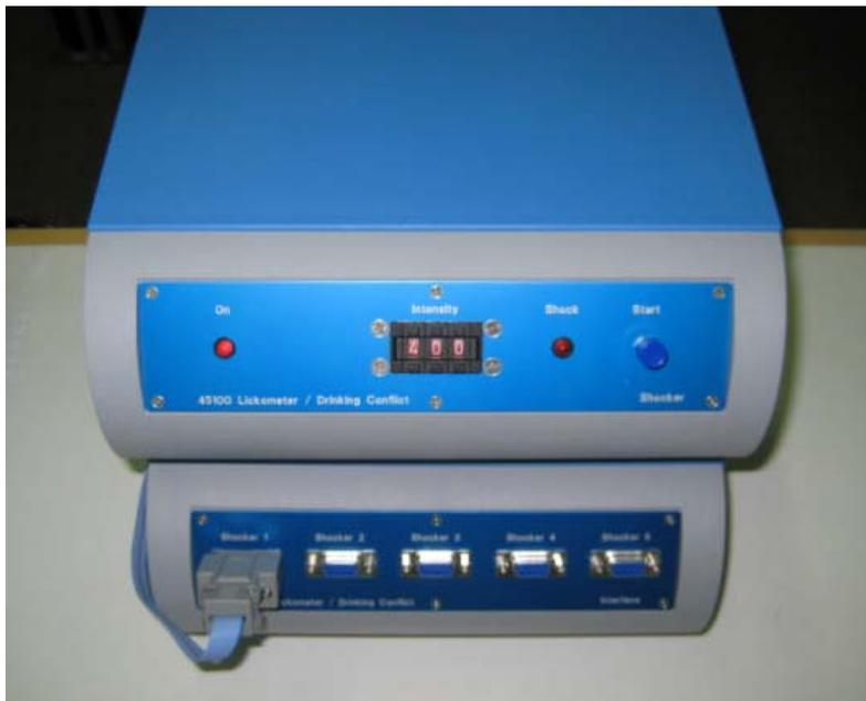
Fig 2: front panel of Shocker (above) and Control Unit (below)
